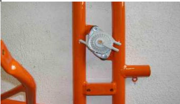
Foto of the frame with the section of the support for the fuel pump (fuel pump mounted)
