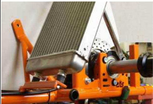
Foto of the frame from the side with the section of the supports for the radiator (radiator mounted)
