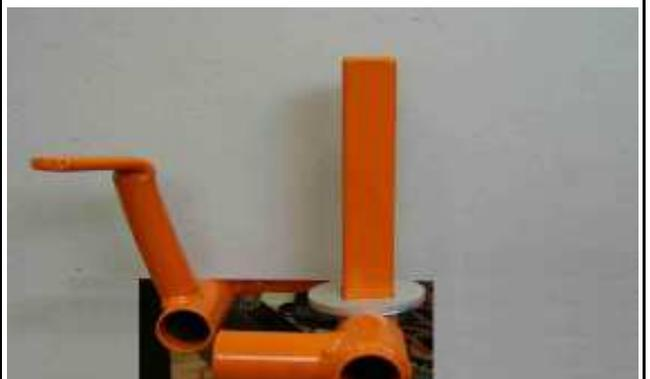
Foto of the frame from the back with the section of the support for the RTPS (Rear Tire Protection System)
