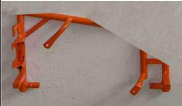
Foto from above of the frame with the section of the two supports for the exhaust system
